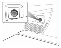
The trunk power socket is located on the right of the trunk. Its maximum operating voltage is 12 V, and its maximum power is 120 W. When the vehicle is powered on, it can be used as power source after opening the cover.
