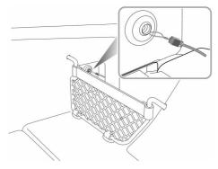
Pull the release cable to unlock the electronic lock, the charging plug can be removed.
