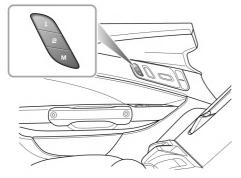
For vehicles provided with the memory function, more extensive personalized settings for driving can be made, i.e., matching the comfort level of the driver seat (seat cushion height, seat fore and aft position, seat back tilt angle, etc.). These personalized settings can be done by operating the switch located on the door (as shown), which can store personalized settings information for up to 2 drivers.
