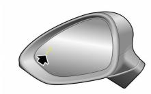
During driving (at a speed over 15 km/h), when the system detects a vehicle running in the blind spot of the rearview mirror of your vehicle or a vehicle approaching behind the adjacent lane, the warning lamp at the corresponding side will illuminate. If the direction indicator lamp at the same side is turned on, the warning lamp will flash, warning the driver that it is dangerous to continue changing lanes.
