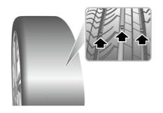
When the tread has worn down to 1.6 mm or below, the indicators will come to the surface of the tread pattern, producing the effect of a continuous band of rubber across the width of the tyre.
