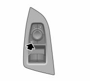
Press the button (arrowed) on the combination switch at driver side, the exterior rearview mirror will be electrically folded. Pushing the button again will return the mirrors to their original position. While unlocking/locking the vehicle, the exterior rearview mirrors will be deployed/folded automatically. This function can be set in the relevant interface in "Vehicle Settings" on the entertainment display.
