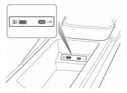
The maximum operating current of the left USB port is 1.5 A, and the maximum operating current of the right USB port is 1.5 A as shown.
