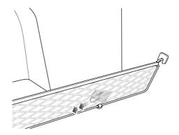
The tailgate cable is located behind the seat, in a carpet hole near the net bag.
