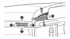
Toggle the knob in the centre of the louvres from side to side to open or close the vent. Direct the air flow by moving the knob up and down, or from side to side.
