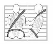
When wearing seat belts, the lap belt section should be positioned as low as possible across your hips (Never cross the abdomen), so that in a collision accident, the lap belt can apply force to the firm hips, reduce the possibility of body moving under the lap belt, and maximize the protection for passengers against injury. This is because if
