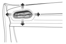
Toggle the knob in the centre of the louvres from side to side to open or close the vent. Direct the air flow by moving the knob up and down, or from side to side.
