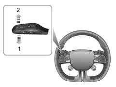
When the vehicle is powered on, move the light lever switch up or down to turn on the turn signal lamp. The corresponding GREEN indicator lamp in the instrument pack will flash when the turn signal lamps are working.
