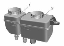
I High Voltage Battery Pack Coolant Expansion Tank
