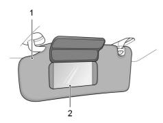
Sunvisor (1) and vanity mirror (2) are arranged on the roof ahead of both the driver and the front passenger.
