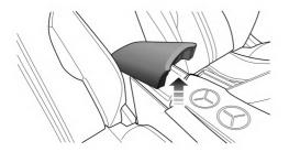
Lift the centre console armrest (as indicated by the arrow) to open the centre console armrest box. Exert little force to put down the centre console armrest to close the centre console armrest box.
