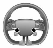
Press the horn button area on the steering wheel (as indicated by the arrow) to operate the horn.
