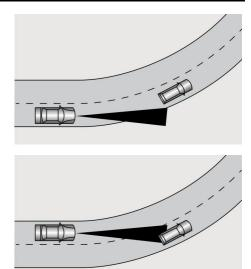
2 If the vehicle ahead changes lane, but not driving into the target lane completely, the ACC may be unable to detect the vehicle.
